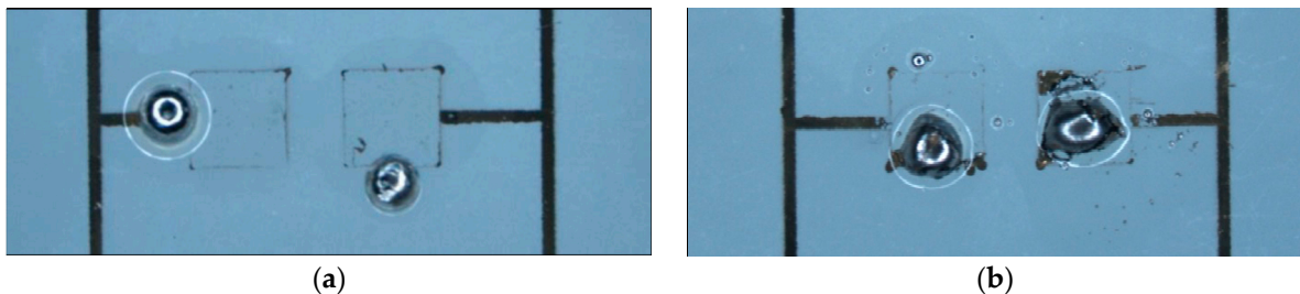
Figure 9. Hot air soldering with SAC solder on printed Ag structures (ink: Sicrys I30 EG-1) on 2D test substrates (Luxaprint 3D mold) at 255 °C (a) and with SnBi solder at 180 °C (b).
