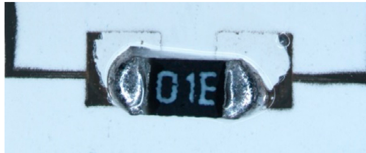
Figure 11. Aerosol jet printed Ag structures with 12 printed layers (ink: Sicrys I30 EG-1) on Luxaprint 3D mold after soldering with SnBi solder in reflow oven with 155 °C peak temperature.
