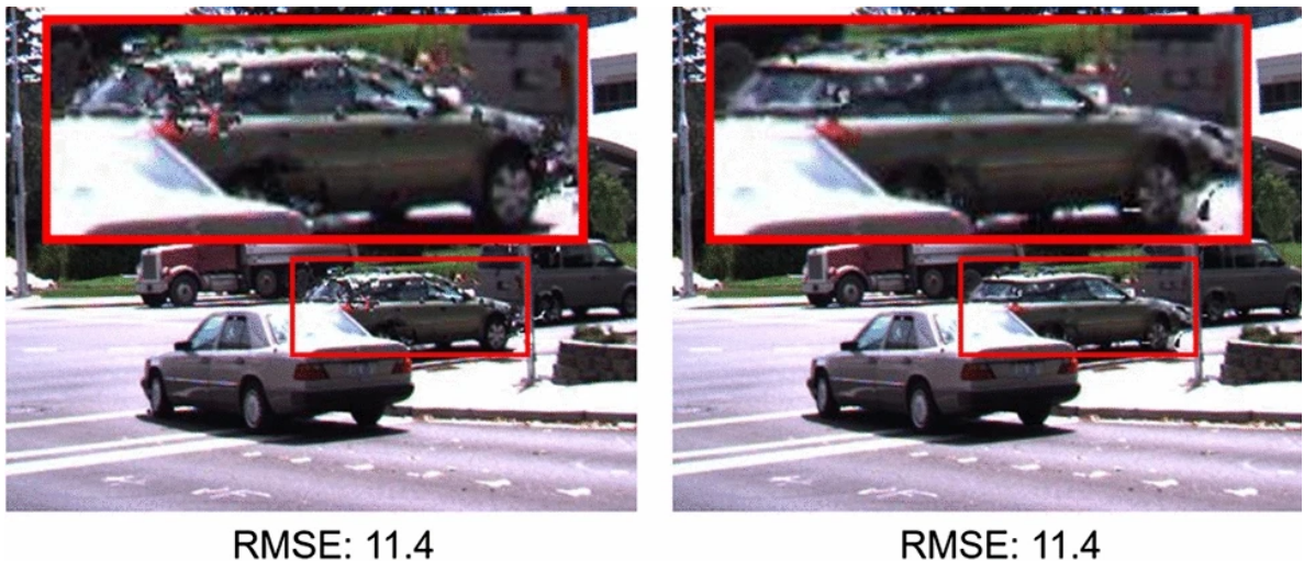
Fig. 5.1: Two frames interpolated with different methods. The RMSE values are equal, but the visual quality differs, in particular in the zoomed regions. Image source: [30]
