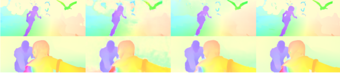
Fig. 2.3: Comparison of flow predictions on two sequences of the Sintel dataset [9]. From left to right : ground truth, VCN [50], IRR-PWC [19], RAFT. Image source [43].
