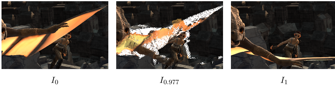
Fig. 3.14: Visualization of artifacts caused by object deformation. On the left and right are the sample frames I_0 and I_1 . In the middle is the result of forward warping for the time step t = 0.977 before inpainting.
