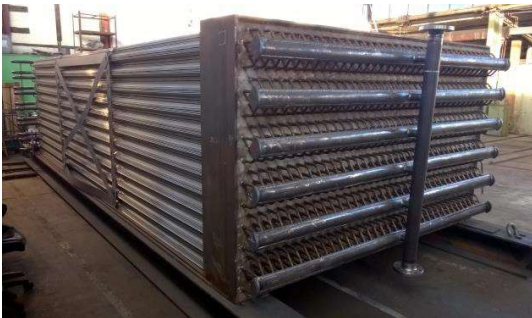
Figure 9: Storage unit build showing complete assembly of the lower header construction.
