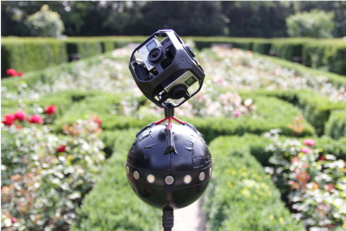
Figure 1.1: The recording setup used to create the audio and video recordings. On the top is the mount with the six GoPros and on the bottom we can see the circular microphone. Picture provided by Miriam Akkermann.
