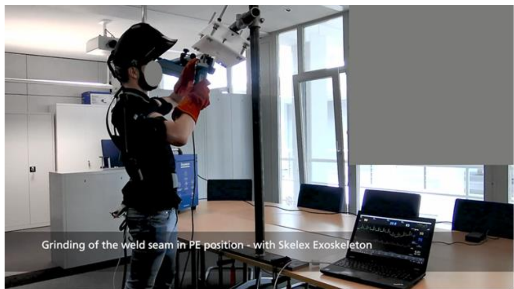
Figure 2. Exemplary illustration of the Position PE during the grinding sequence. Fraunhofer IPA.
