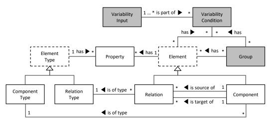
**Figure 4.** Class diagram of VDMM based on EDMM (EDMM original classes in white, added classes for variability in grey).
