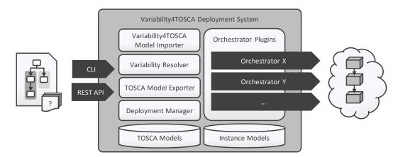
Figure 5. System architecture of a Variability4TOSCA Deployment System.
