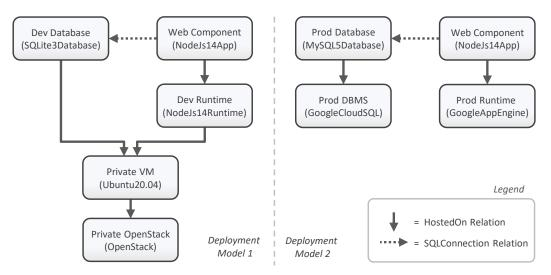
**Figure 1.** Two different deployment variants for the motivating scenario: deployment model 1 for development (**left**) and deployment model 2 for production (**right**).
