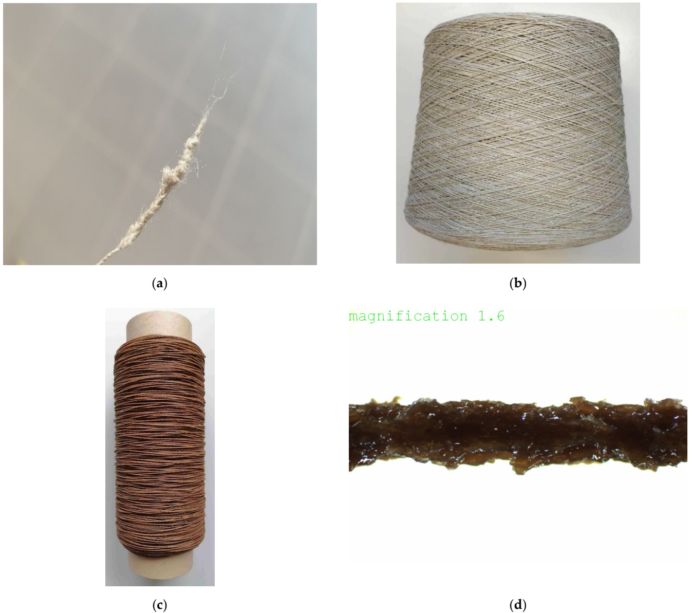
Figure 2. (a) Example of breakage in flax yarn; (b) bobbin of flax yarn (FL) without coating; (c) bobbin of flax yarn with lignin (FL-LI coated yarn); (d) close-up view of FL-LI coated yarn (the magnification is 1.6).
