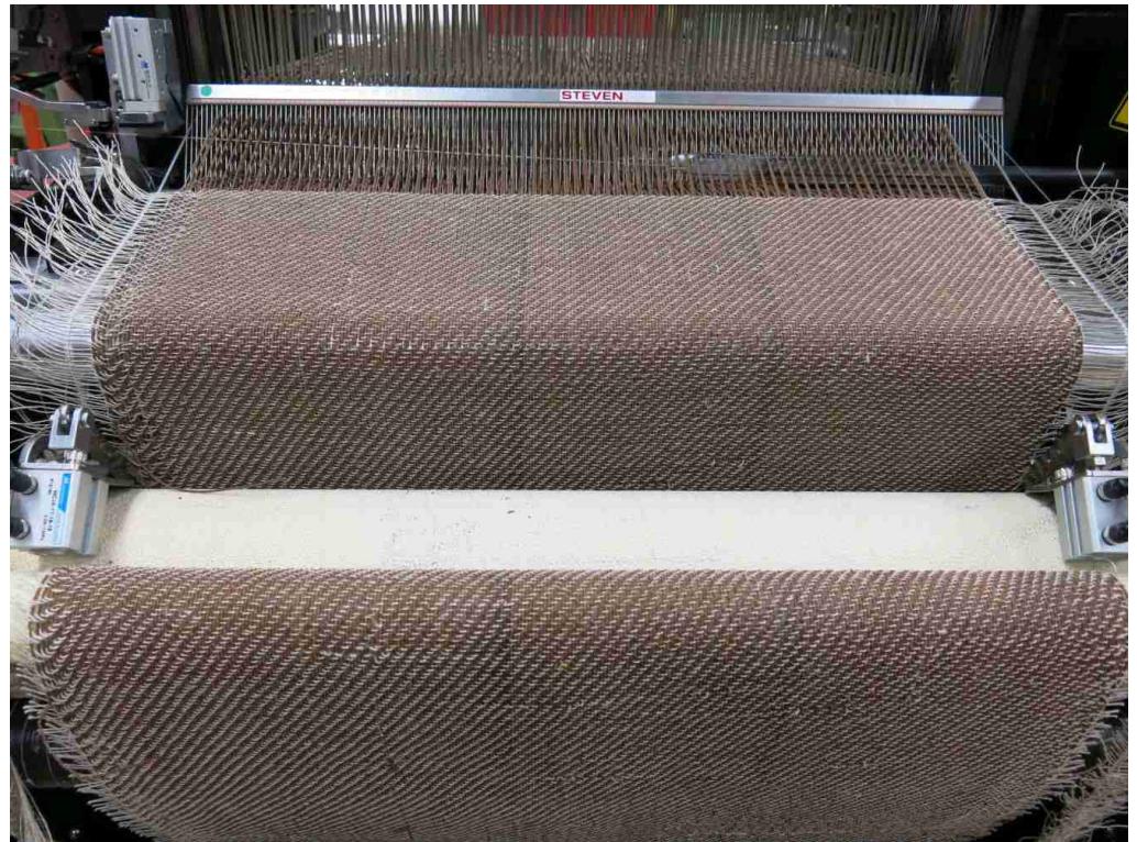
Figure 3. Weaving with FL-LI coated yarn (warp) and FL commercial yarn (weft).
