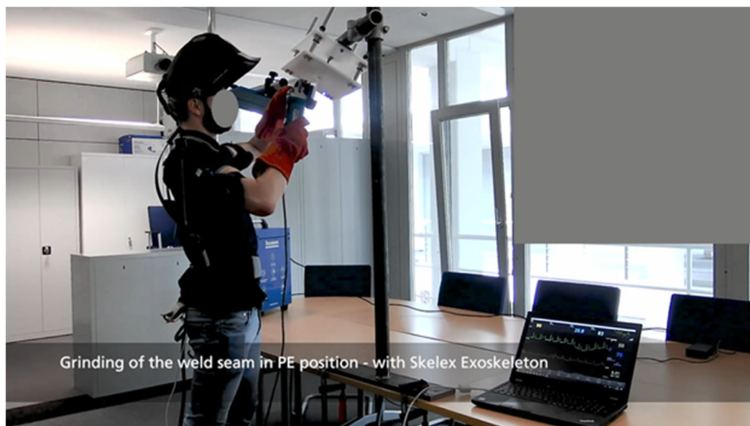
Figure 2. Exemplary illustration of the PE Position during the grinding sequence | Fraunhofer IPA.
