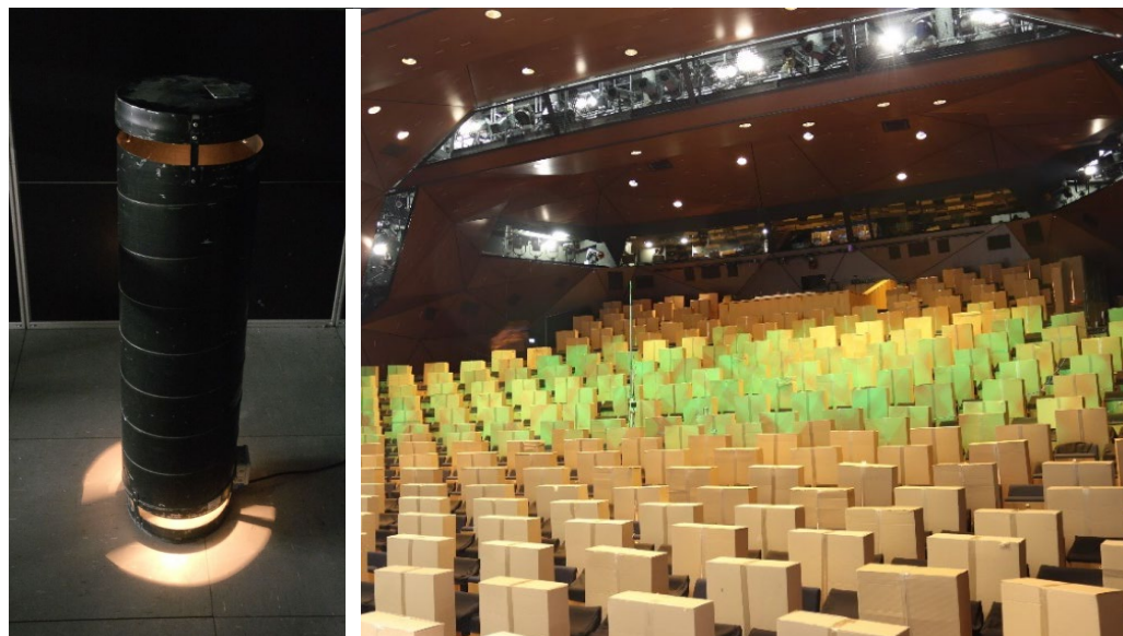
Figure 3. Professional thermal person dummy (left), low cost variants in Stuttgart Drama Theatre (right).
