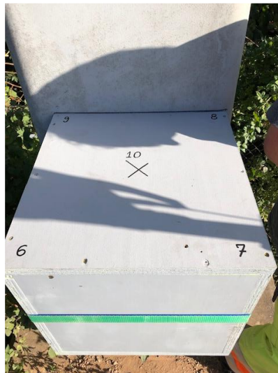
Figure 8. Reference box used for spatial synchronisation of multitemporal laser scans.
