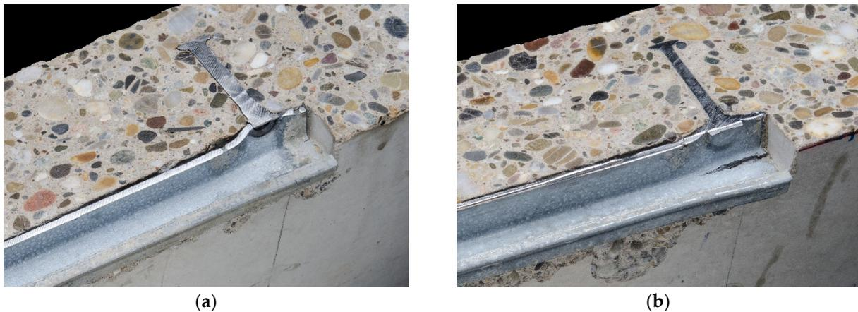
**Figure 3.** Photographs of typical failure modes for anchor channels in fatigue tension tests: (a) Steel failure of connection anchor channel; (b) Steel failure by crack formation in the channel flange.
