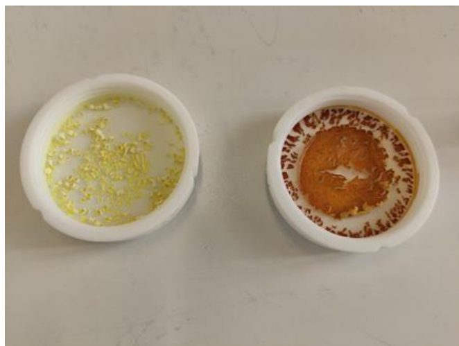
Figure IV-5. No film formation after evaporation of the solvent
