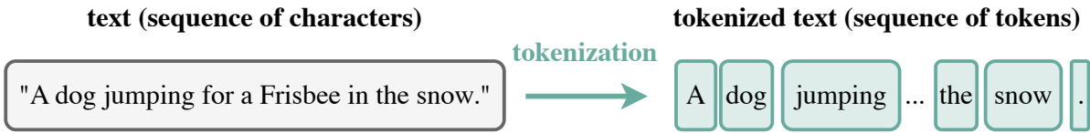
Figure 2.3.: Tokenization maps a text string to a sequence of tokens. Tokens can be (sub)words or punctuation.
