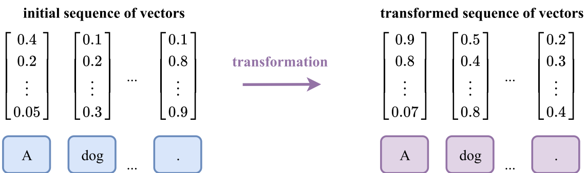
Figure 2.5.: Each token's vector representation is transformed into a contextualized vector representation.
