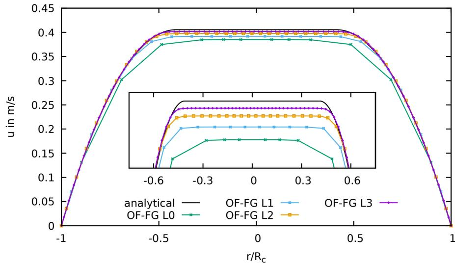
Figure S4: Velocity profiles for different mesh refinements modeled with the software OpenFOAM (FG). The data is shown for the bi-viscous model in the  $cv$  case. The lines connect the numerical points as guidance of the eye. The plug-flow region is also shown enlarged for  $u = 0.37 - 0.41 \text{ m s}^{-1}$ .
