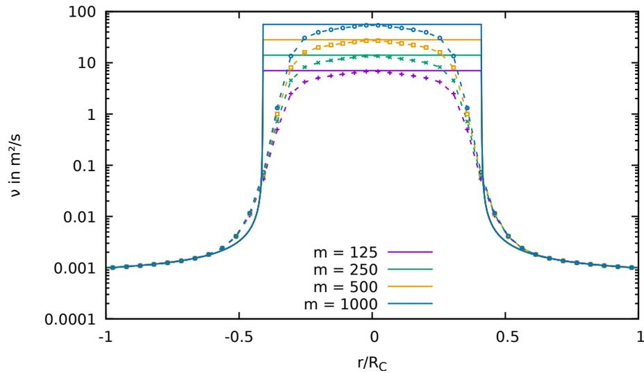
Figure S8: Viscosity profile  $\nu(r)$  for different regularization parameters  $m$  in the OpenFOAM solution for the Papanastasiou model ( $cv$ ). The analytical solution is drawn as continuous lines, the numerical results at the center of the grid cells are shown as points. The dashed lines connect the numerical points as guidance of the eye.
