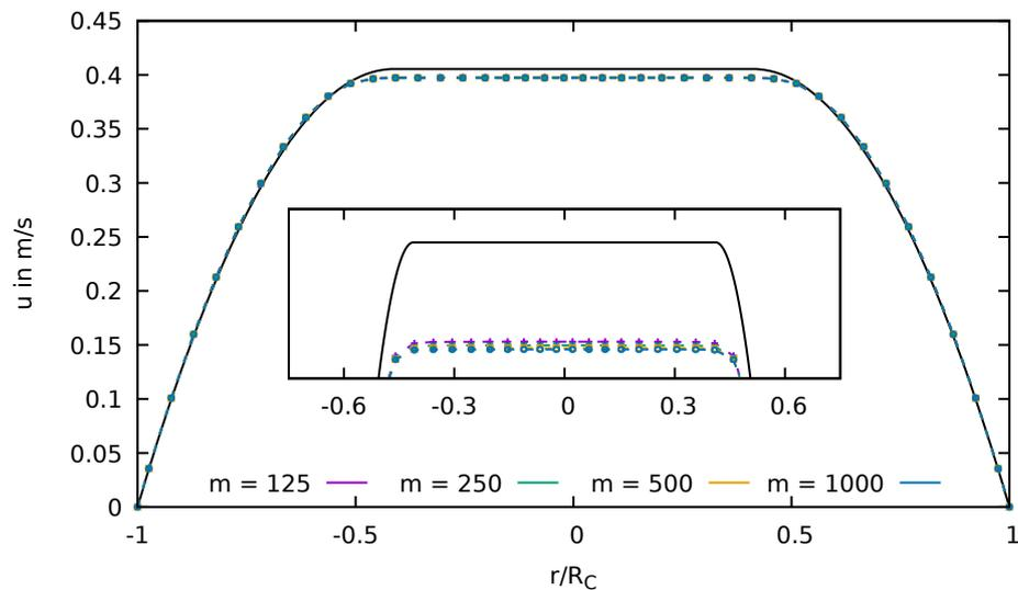
Figure S7: Velocity profile  $u(r)$  for different regularization parameters  $m$  in the OpenFOAM solution for the Papanastasiou model ( $cv$ ). The analytical solution is drawn as continuous lines, the numerical results at the center of the grid cells are shown as points. The dashed lines connect the numerical points as guidance of the eye. The plug-flow region is also shown enlarged for  $u = 0.395 - 0.408 \text{ m s}^{-1}$ .
