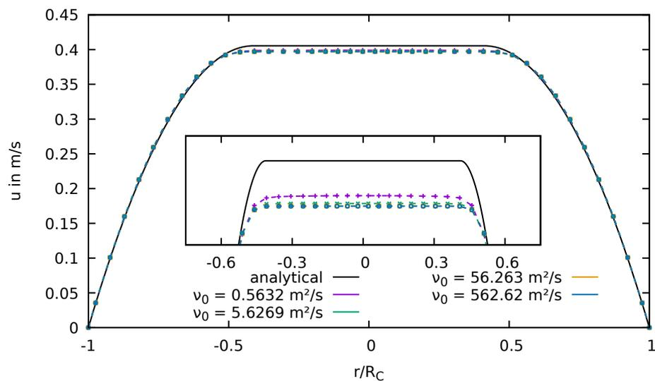
Figure S5: Velocity profile  $u(r)$  for different regularization parameters  $\nu_0$  in the OpenFOAM solution for the bi-viscous model ( $cv$ ). The analytical solution is drawn as continuous line, the numerical results at the center of the grid cells are shown as points. The dashed lines connect the numerical points as guidance of the eye. The plug-flow region is also shown enlarged for  $u = 0.39 - 0.41 \text{ m s}^{-1}$ .
