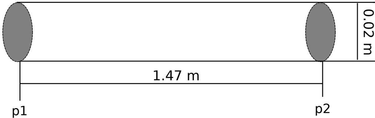
Figure S1: Setup of the cylindrical simulation geometry of length 1.47 m and diameter of 0.02 m. The pressure drop is calculated between the pressure sensors p1 and p2. The suspension flows from left to right.
