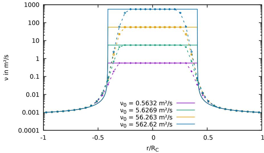
Figure S6: Viscosity profile  $\nu(r)$  for different regularization parameters  $\nu_0$  in the OpenFOAM solution for the bi-viscous model ( $cv$ ). The analytical solution is drawn as continuous lines, the numerical results at the center of the grid cells are shown as points. The dashed lines connect the numerical points as guidance of the eye.
