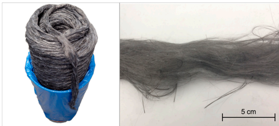
Figure 6. Sliver coil (left) and texture of the recycled staple fiber sliver (right).
