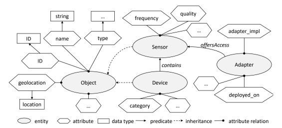
Figure 2. Example of an ontology-based model for IoT environments based on [11].
