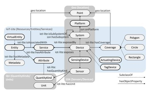
Figure 4. IoT-Lite ontology (based on [23]).
