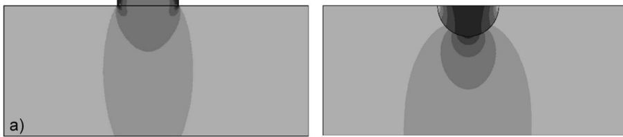
Fig. 5 Elastic stress distribution depending on punch geometry [10]: a) flat punch, b) punch with convex shape
