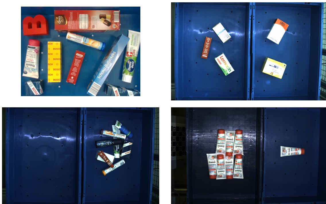
Figure 4.9: Example of evaluation datasets. The top-left image shows an example from the RealSense dataset, while the top-right image displays a simple evaluation sample from the Zivid dataset. The bottom-left image illustrates a typical bin containing overlapped random objects from the Zivid dataset, and the bottom-right image presents a special case where objects are stacked side by side from the Zivid dataset.
