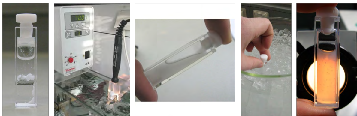
Fig. 6.1 Preparation of a gelled microemulsion sample. From left to right: cuvette with all components; heating of the sample in the water bath; mixing the sample in the sol state; gelling the sample in the ice bath; check of the gelled sample's homogeneity.
