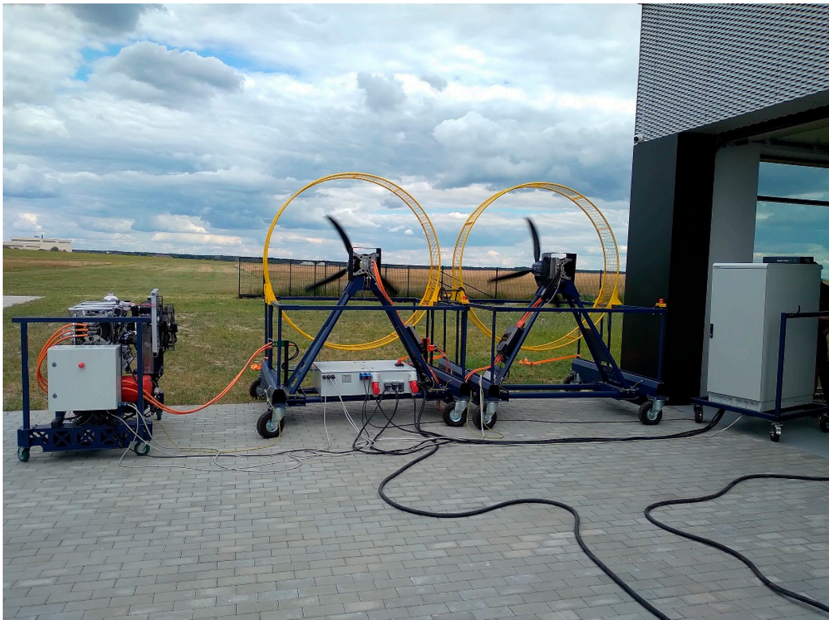
Figure 13. Ground testbed of the PW-X20 propulsion system.
