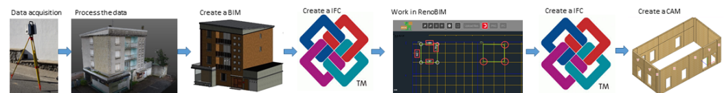
Figure 4. Process proposed for RenoBIM in BERTIM.
