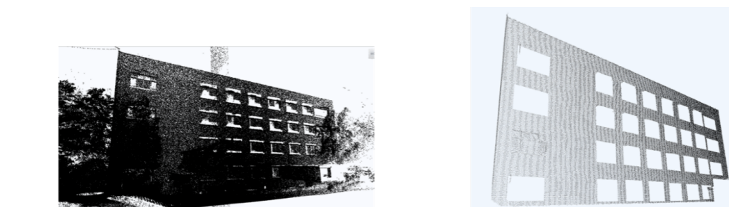
Figure 8. (Left) Merged Point Cloud of a building and surrounding area. (Right) After processing.
