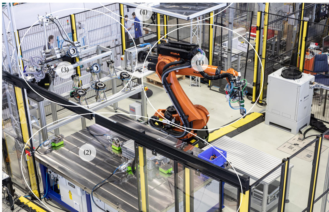
Figure 9. DeMoBat disassembly station to extract modules from packs: (1) robot, (2) processing table, (3) tool station, and (4) vision system. © Fraunhofer IPA/Photo: Rainer Bez. Own representation.
