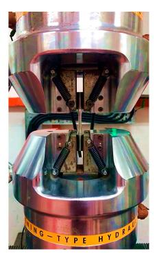
Figure 4. Specimen during the fatigue test.
