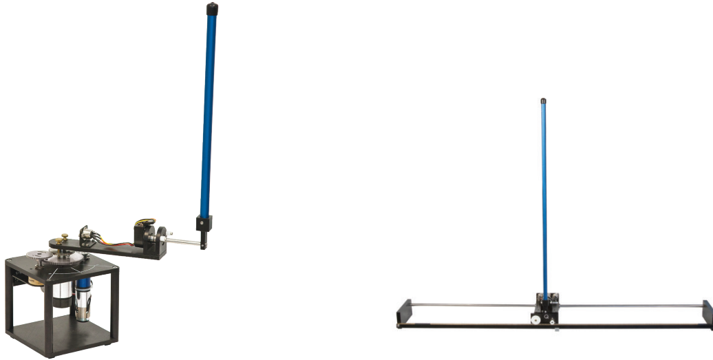
(a) The rotary inverted pendulum by Quanser [Quab] (b) The cartpole inverted pendulum by Quanser [Quaa]
