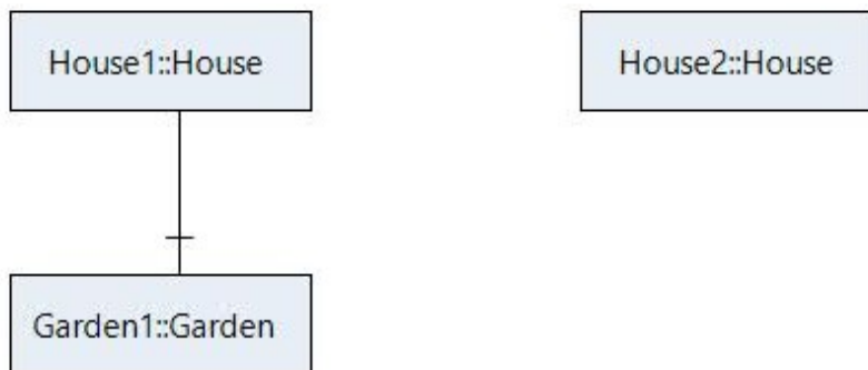
Figure 3.4: All possible variations of Instances for the House ObjectType in figure 2.2, using a complete interpretation of OPC UA models.
