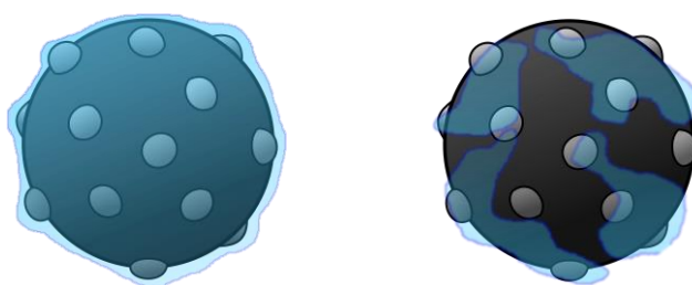
Figure 3 Illustration of Pt/C particle fully or partially covered with \text{SiO}_2
