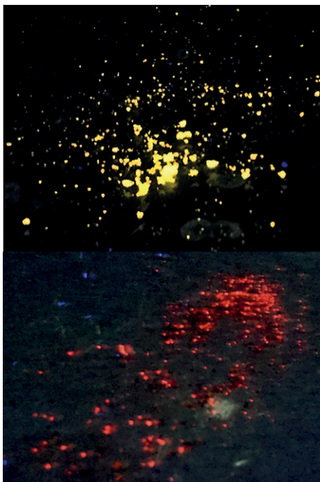
Figure 10. Luminescence of \text{Li}_2\text{Eu}_3\text{Br}_2[\text{BO}_3]_2 (top) and \text{Eu}_3[\text{BO}_3]_2 (bottom) under UV light ( \lambda = 254 \text{ nm} ).
