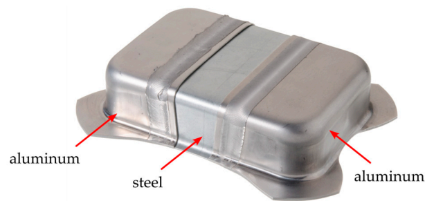
Figure 2. Deep-drawn friction stir-welded aluminum–steel hybrid.
