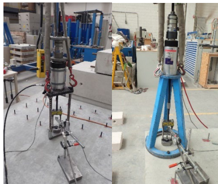
Figure 3. Confined and unconfined test setup.
