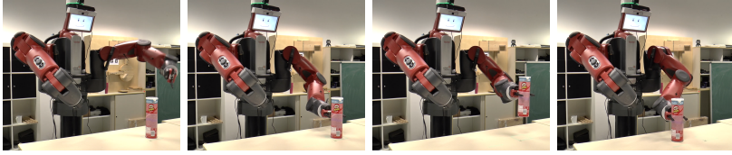
Figure 3.1: Baxter robot performing pick and place (a chain of reaching tasks)
