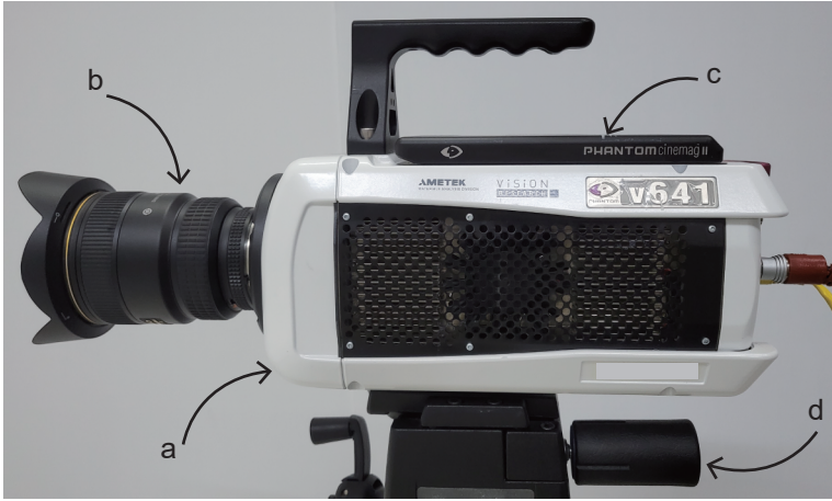
Figure 1.13.: High-speed camera to observe detailed behavior of the robot. a camera body (V641, PHANTOM), b. lens, c. Memory, d. tripod
