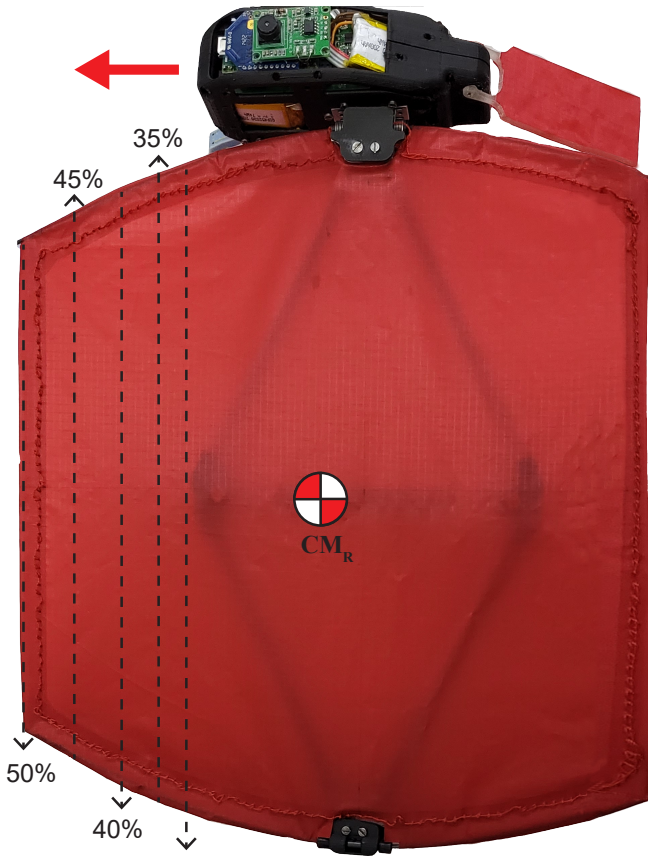
Figure 1.4.: Configuration of the airfoil. Red arrow denotes gliding direction. Black-dotted arrows denote leading edge of the different locations of the robot's center-of-mass ( CM_R ). The 30% to 50% denote locations of CM_R of the chord length measured from the leading edges. The mark of the CM_R is represented on the wing.
