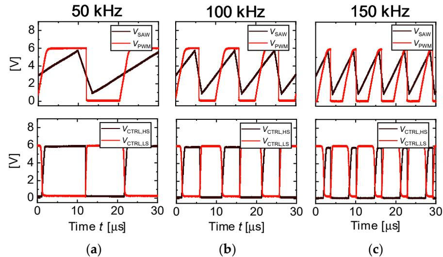
**Figure 5.** Measurement of the PWM generator and dead time control with the three different carrier frequencies (a) 50 kHz, (b) 100 kHz, and (c) 150 kHz at the same operating point ( $V_{\text{FB}} = 2.66$  V and  $V_{\text{REF}} = 2.95$  V).
