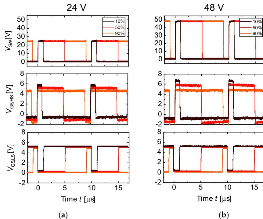
**Figure 4.** Switching characterization of the driver ( $V_{SW}$ ,  $V_{PWM,HS/LS}$ ) with an input voltage of (a) 24 V and (b) 48 V at  $V_{DD} = 6$  V,  $f_{SW} = 100$  kHz, and three different duty cycles  $DC = 10/50/90\%$ .
