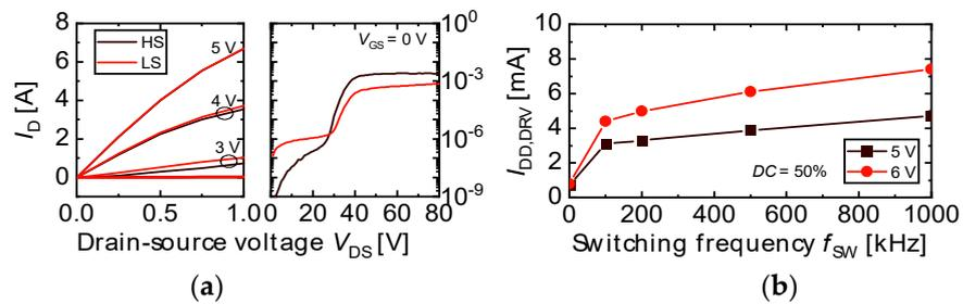
**Figure 3.** (a) Output and breakdown characteristic for HS/LS transistor and (b) driver current  $I_{DD,DRV}$  as a function of the switching frequency with  $V_{DD} = 5/6$  V and  $DC = 50\%$ .
