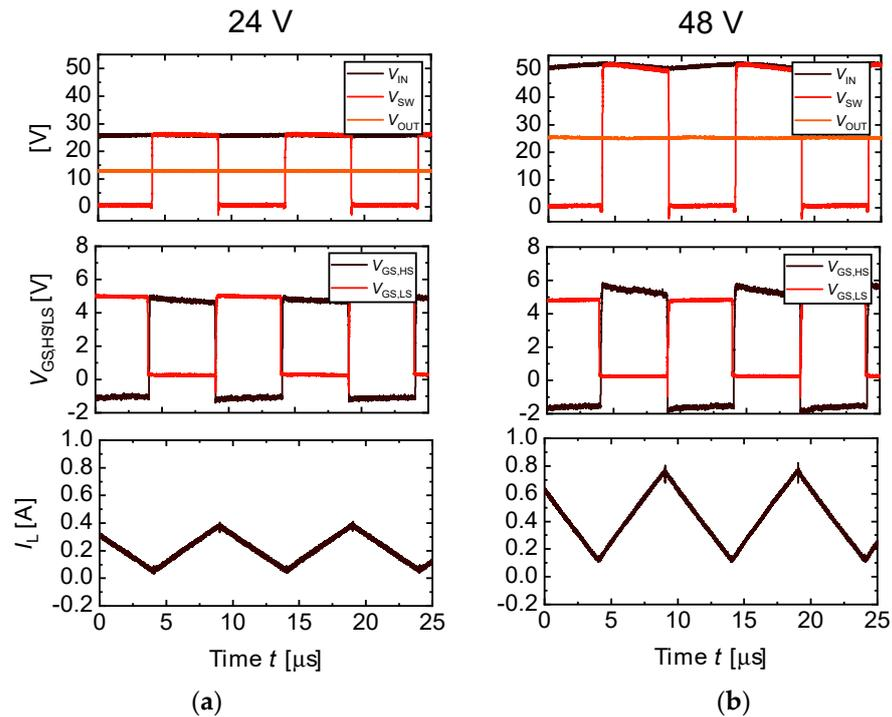
**Figure 6.** Switching characterization of the DC–DC converter ( $V_{IN}$ ,  $V_{SW}$ ,  $V_{OUT}$ ,  $V_{GS,HS/LS}$ ,  $I_L$ ) with an input voltage of (a) 24 V and (b) 48 V at  $V_{DD} = 6$  V,  $f_{SW} = 100$  kHz, and load of  $24 \Omega$ .
