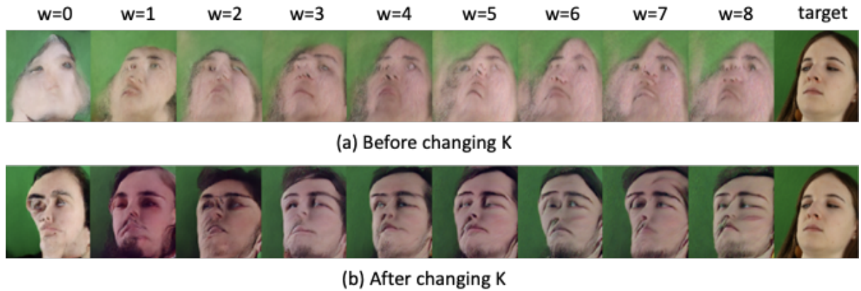
Figure 5.1: Comparison of the results in accordance with the change in intrinsic matrix. In both cases, the conditions are (R, T, K) . (a) shows the results using the original intrinsic matrix from the preprocessed dataset, i.e., image size of 512. (b) shows the results after changing the intrinsic matrix to our image size setting of 128. The labels denoted as w is the hyperparameter that controls the strength of the conditioning information.
