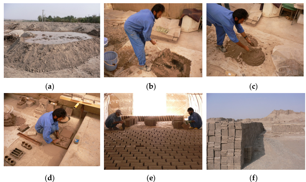
Figure 1. Adobe production: (a) adding water to soil and leaving for one or two days, (b) mixing adobe components using a shovel, (c) mixing adobe components by hand, (d) forging in the mould, (e) trimming and placing the adobe units vertically for drying faster, (f) dried adobe units ready to be used in construction, Bam citadel, 2007.
