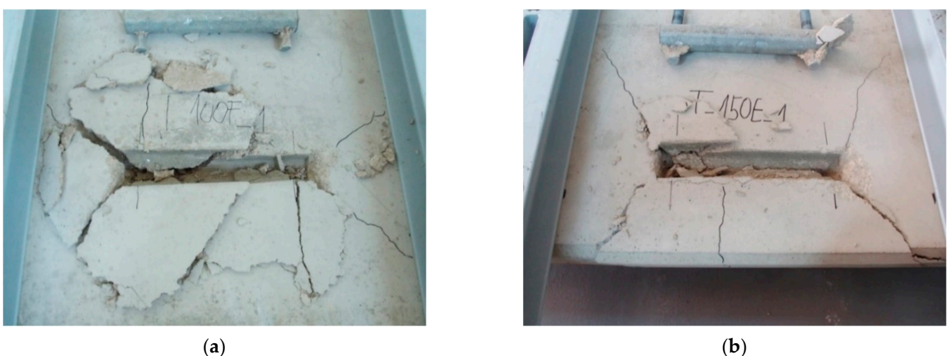
Figure 11. Breakout patterns: (a) in-field installation— h = 100 mm; (b) installation near the edge— c_1 = 150 mm.
