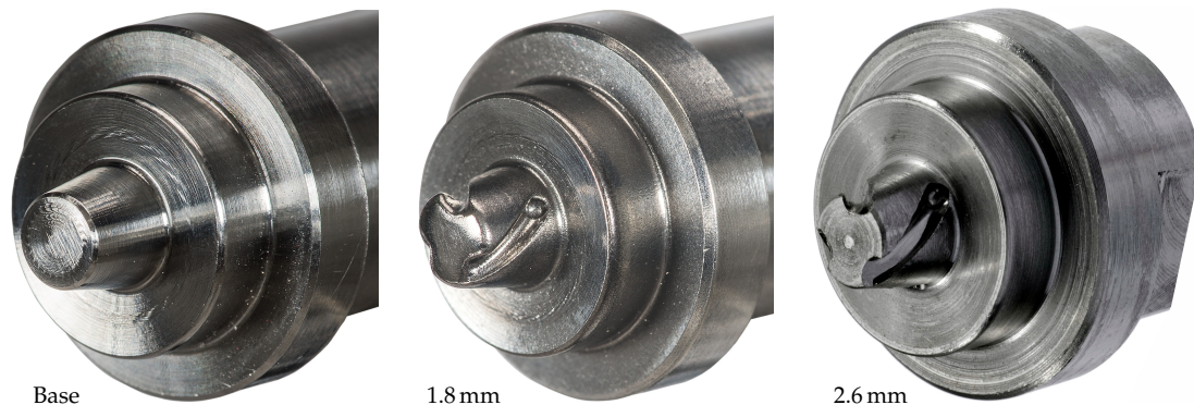
Figure 7. Development stages of the tools manufactured for verification. Base geometry without contouring, third and fifth design iterations with 1.8 mm and 2.6 mm structure width, respectively.
