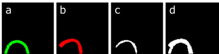
Figure S5 Visualization of the Jaccard index calculation steps (a) Simulated frame, F_{sim} , (b) actual frame, F_{exp} , (c) intersection of frames, F_{sim} \cap F_{exp} , and (d) union of the frames, F_{sim} \cup F_{exp} .
