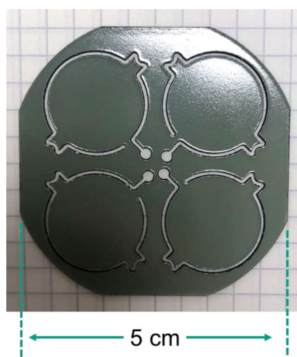
Figure S7. The MS-PCC (type II) sample photo after PLD process.
