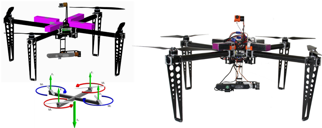
Figure 13. Basic structure of a multicopter, its CAD model and its concrete realization.
