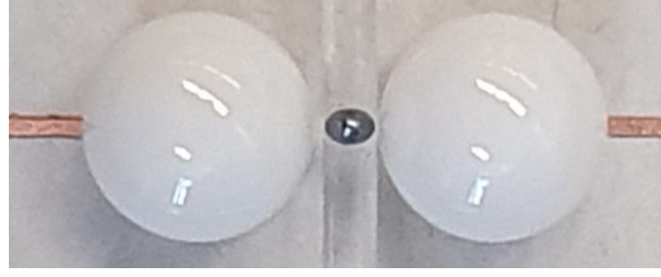
FIGURE 3.32: Setup 2 at 30 GHz 0.4 mm silicon particle in tube filled with water.
