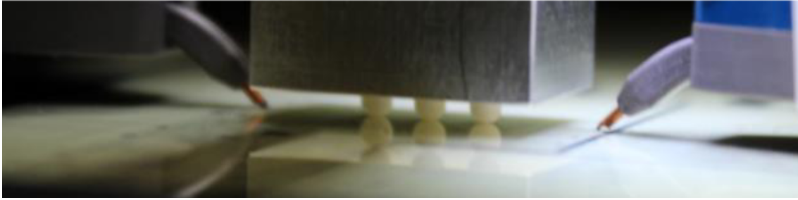
FIGURE 2.9: SDR with three between chip and metal cover sandwiched alumina ceramic spheres at 65 GHz [10].
