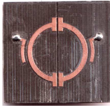
FIGURE 2.1: SRR with double capacity split 3 GHz [2].
