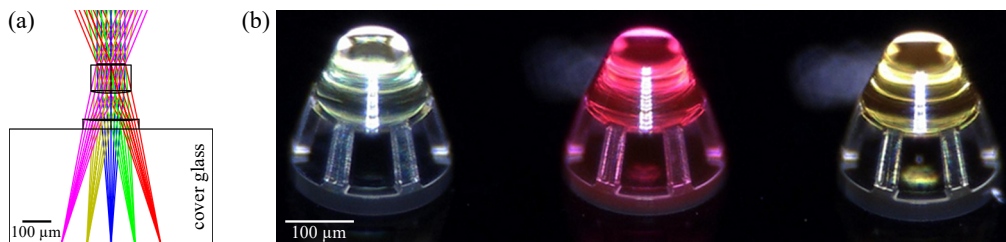
Fig. 1. Colored micro-optics. (a) Optical design of the lens system. (b) Microscope image of multiple micro-optics of different color printed successively on the same glass substrate.
