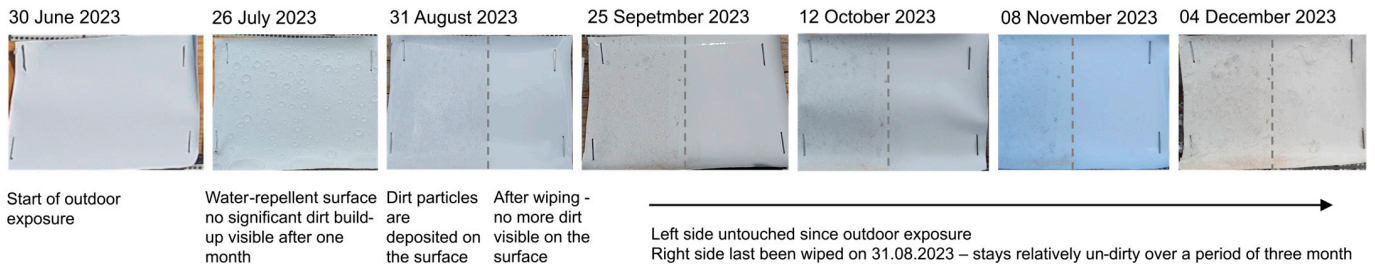
Figure 11. Longevity measurement. Sample: PES g/m 2 coated (total coating thickness: 250 ± 20 μm).
