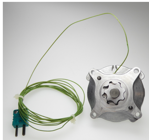
Figure 9. Gerotor pump with additional temperature sensor in gap between outer gear and pump housing.
