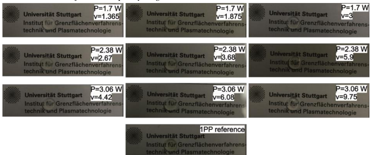
Figure SI 14: Representative photos of hydrogels prepared by 2PP curing and after swelling to equilibrium.
