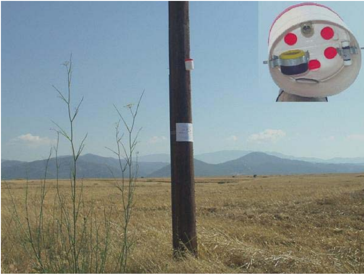
Annex A.1. Shelter with diffusive sampler used in the field
