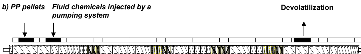
Fig. 2.2.1: Screw configuration used for the functionalization processes (ZSK30)
