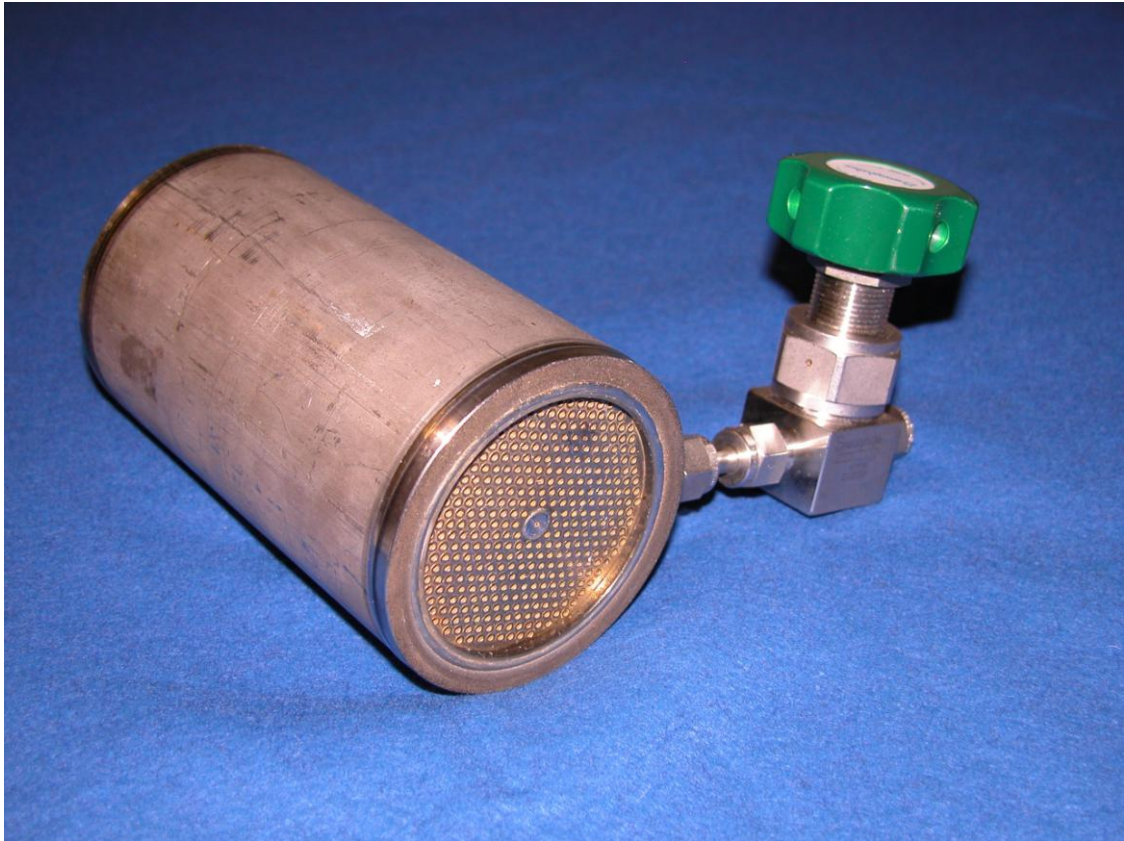
Figure 2-10: Capillary tube bundle reaction bed
