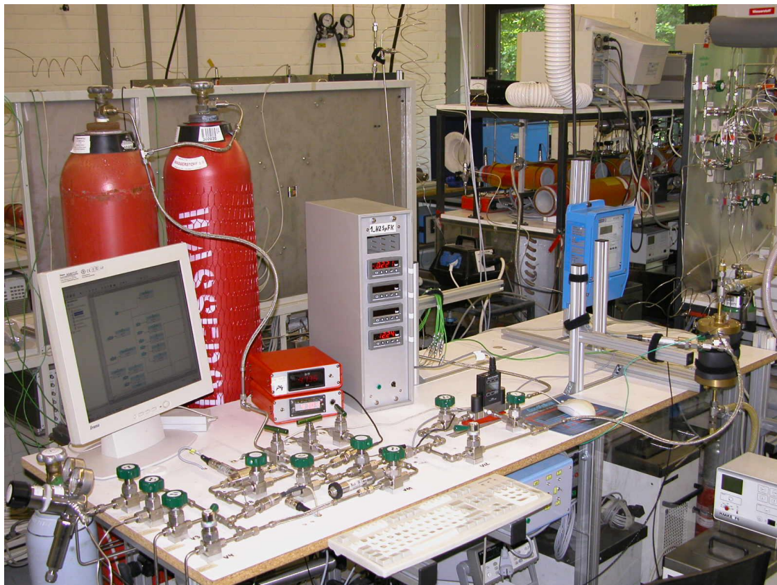
Figure 2-2: Test bench for reaction bed dynamics measurements
