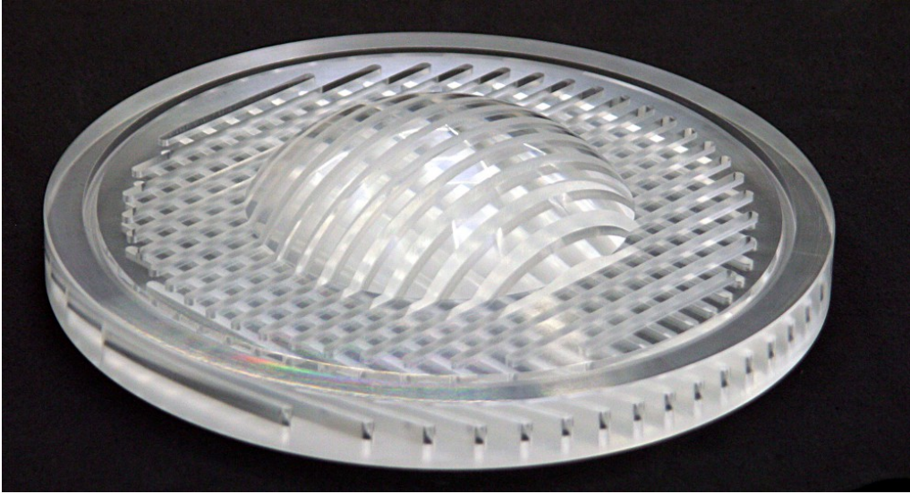
Figure 4.6: Microwave lens made of PMMA acting as vacuum transition for the 8 GHz heating system.
