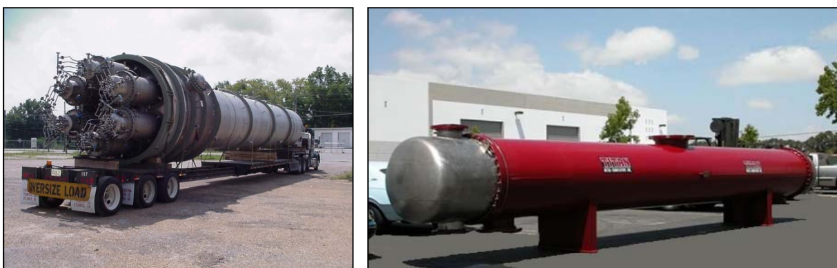
Figure 1.1: Left: shell and tube heat exchanger made by Addison Fabricators Inc., Addison, Alabama, USA (8000 tubes/90 tonnes). Right: titanium shell and tube heat exchanger made by TITAN Metal Fabricators, Camarillo, California, USA (1.07 m shell outside diameter, 7.3 m maximum length, 25 tonnes, 1282 tubes).
