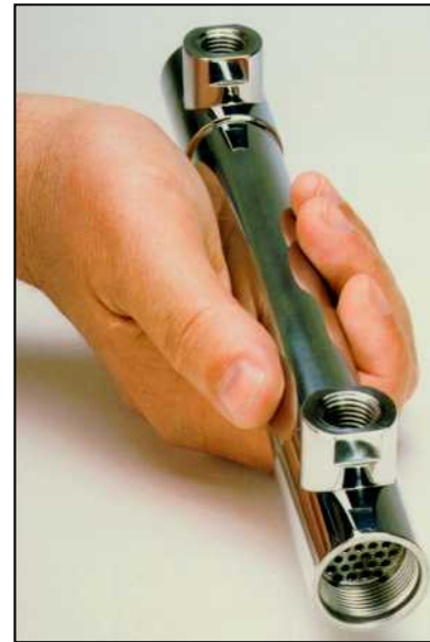
Figure 1.2: Shell and tube heat exchanger for temperature control systems made by Exergy LLC (inside shell diameter = 22.5 mm, maximum length = 248 mm and tube number = 24)
