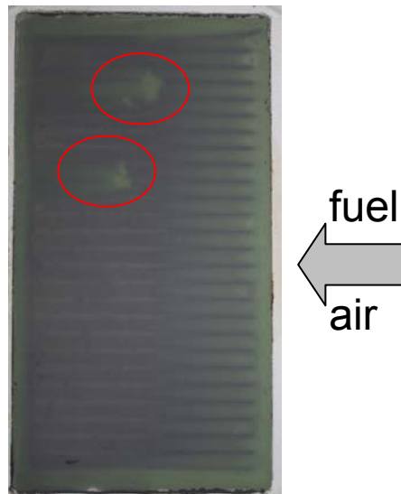
Figure 8-12: Partially oxidised anode after operation at 700 mV total cell voltage. Strongly oxidised areas in the middle correspond to segments 11, 14 and 15.
